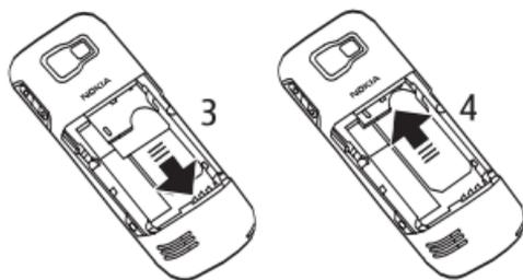
6. Follow step 3 and 4 of 'Install the SIM card and battery' to replace the battery and the back cover.
